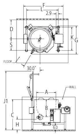
\*Dimensions on these drawings are applicable when using an optional 2" diameter draw-off valve. If a 3" diameter draw-off valve is required, contact AccuTemp for applicable dimensions.
