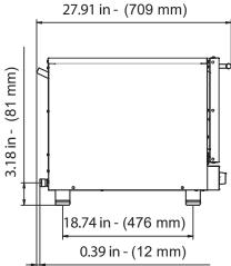
\* Oven must be installed a minimum of 19.7" (500 mm) from any significant source of heat and/or grease (for example: fryers, burners, kettles, open flames, etc.)
