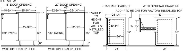
Note: Available with compressor left or right. Compressor left model shown.
